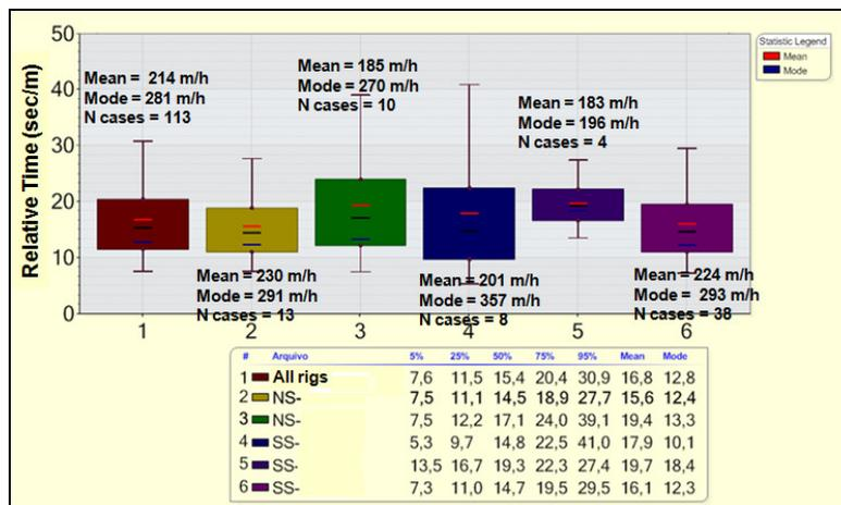
**Figure 5:** Box Plot graph of relative time (sec/m) obtained in the trip-in operation in an open well, for all rigs (case 1) and each rig individually (case 2 to 6). The data collected to generate this graph is used in the operational monitoring shown in Figure 6.
