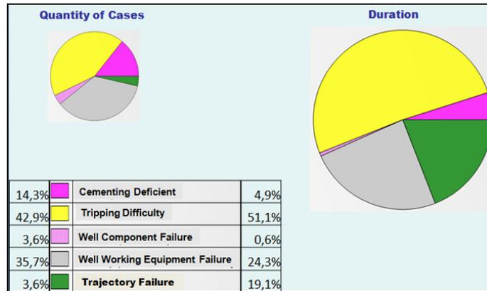
**Figure 9:** Abnormal Occurrences, by number of cases and by duration for the Surface Phase in Slender Wells. One can see that Tripping Difficulty (in yellow) is among the greatest impact, not only by duration but also per number of cases.
