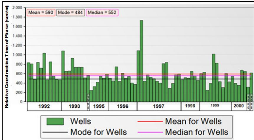
Figure 7: Relative Construction Time of Directional Production Phase 9 5/8".
