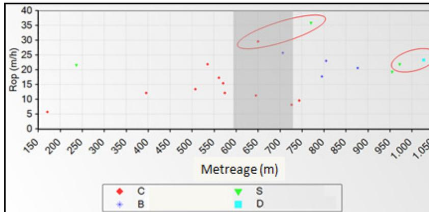
**Figure 12:** Graph showing ROP x Length drilled, classified by bit manufacturer, for 17½” tricone bits. Note that the bit from manufacturer S presented the highest ROP and the second in longest drilled length, while manufacturer D had the longest drilled length and manufacturer C had the highest ROP in the mean length of the phase (shown in the darker stripe on the graph).
