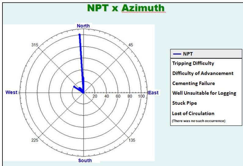
**Figure 10:** NPT x Azimuth for the correlation wells, indicating the incidence of abnormalities in the direction N5W that, if possible, should be avoided in the drilling of the new well.
