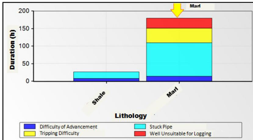
**Figure 3:** Graph showing non-productive time x lithology. This figure was obtained from the records of occurrence of Difficulty of Advancement, Tripping Difficulty, Stuck Pipe and Well Unsuitable for Logging, its duration, and the lithology where each abnormality occurred in the various correlation wells.
