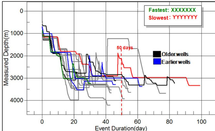
**Figure 2:** Comparison of the Time x Depth curve of the wells in the field made with the technology of construction of pilot well + horizontal. The green line is the fastest while the red is the slowest well in this set.
