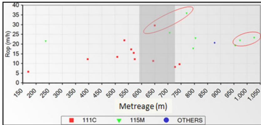
**Figure 11:** Graph showing ROP x Length drilled, for each IADC code applied, for 17½” tricone bits. Note that the IADC code 115M presented higher ROP for the longest drilled length, while the IADC code 111C had the highest ROP in the mean length of the phase (shown in the darker stripe on the graph).
